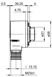
Through hollow shaft, flange socket M23
